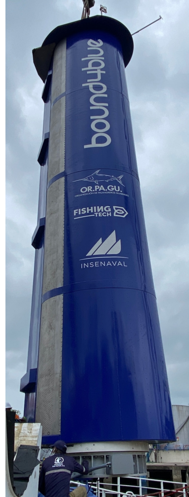
First eSAIL® unit ready for installation (Left: our facilities in Spain / Right: Shipyard in Panama)
