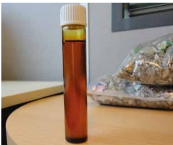
A sample of DieselR, the synthetic diesel fuel produced from waste fractions
