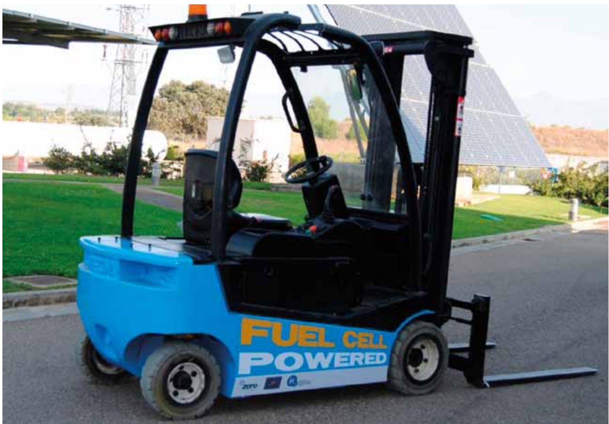
One of the zero emission hydrogen-fuelled vehicles at the site in Walqa
