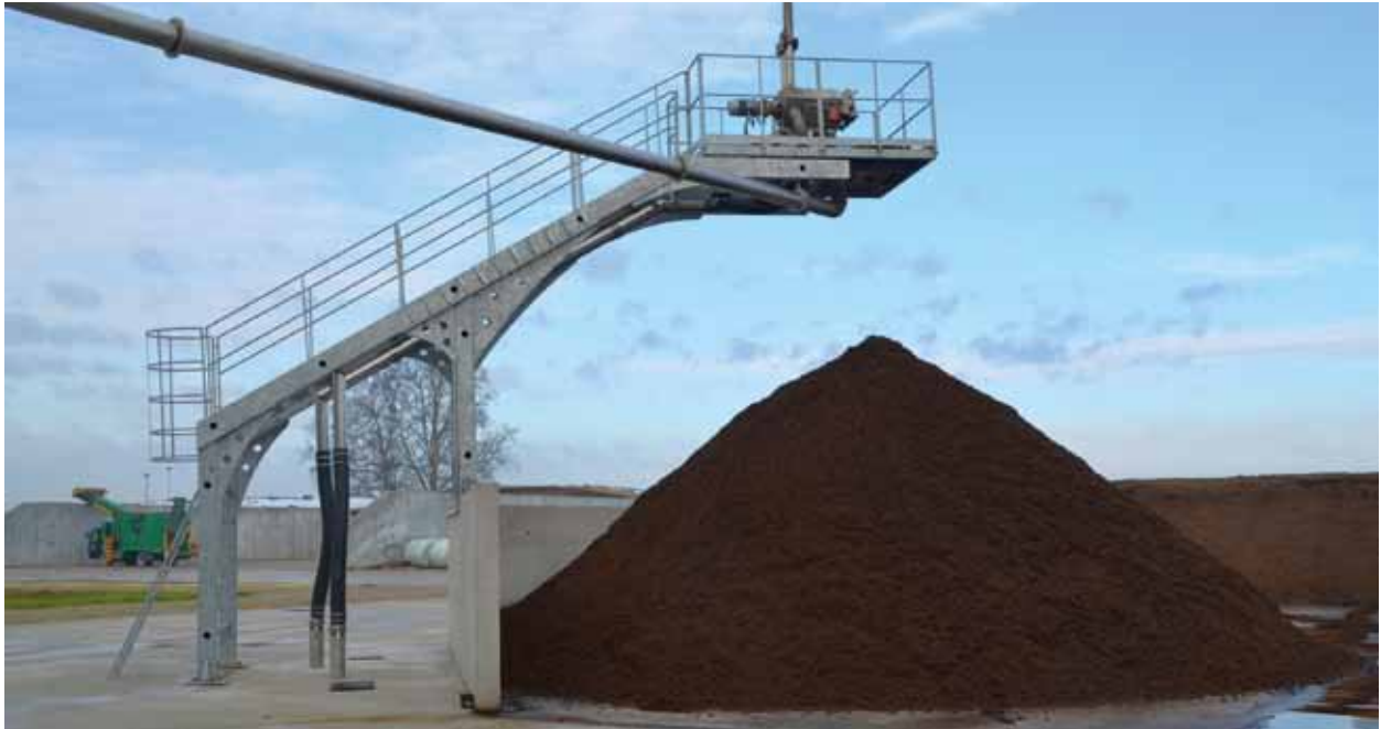
The mobile solid-liquid separator that creates clarified liquid slurry and dry fractions
