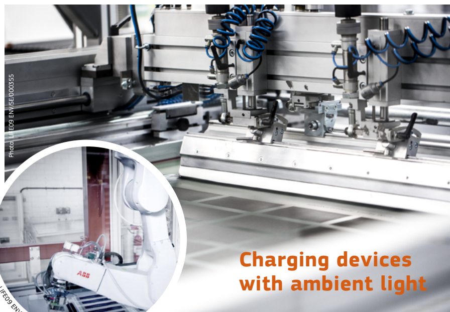
Screen printing the innovative solar cell technology
