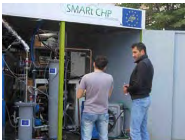
Using less than 2 kg/h of biomass and a small amount of propane the pilot plant can generate approximately 3 kW el of electrical power and 8 kW of thermal power
