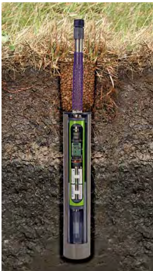
Probes buried in the soil capture and count the microfauna
