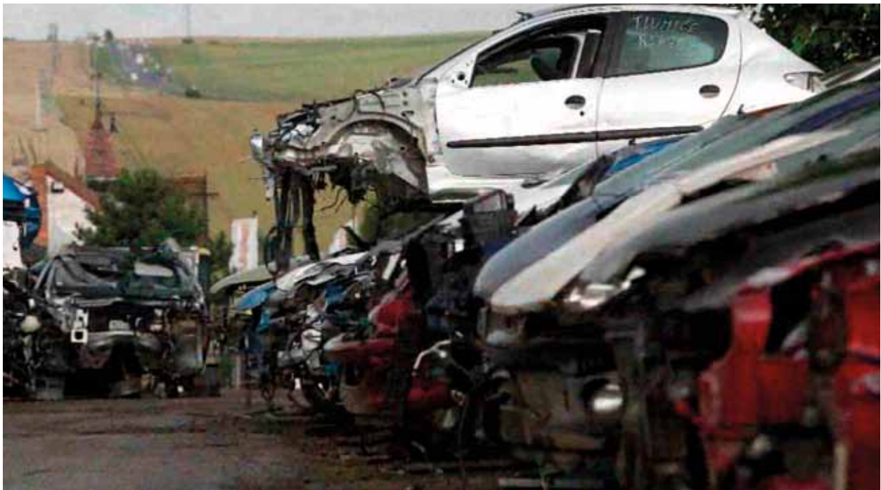
The project treated 1 tonne of ELV waste per hour, breaking vehicles into valuable and reusable parts
