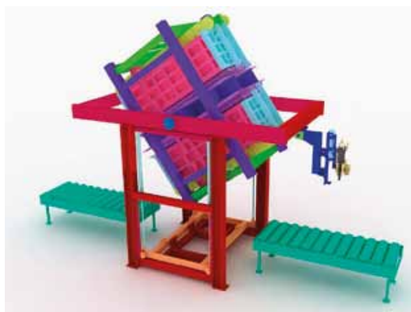
The new insulation process is also time-efficient as it enables two fridges to be processed at once
