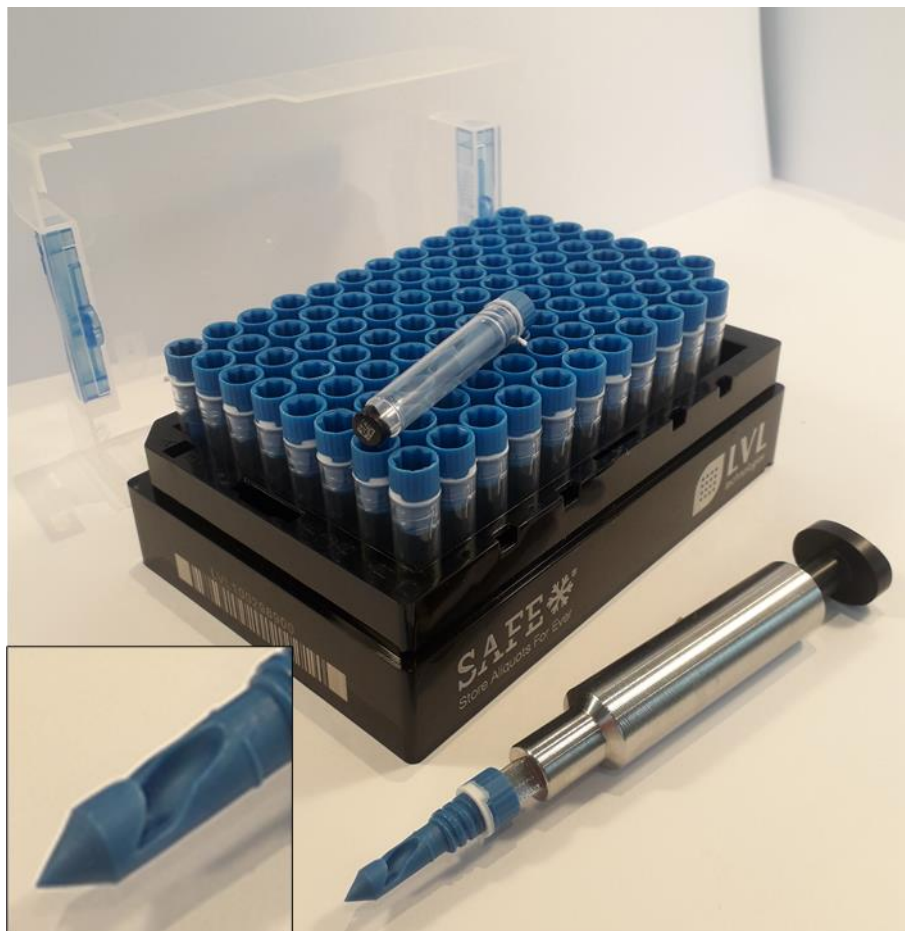
Figure 7.1. The LVL Technologies SAFE® genetic sampling system. A close up of the tissue collection window is shown in the inset.
