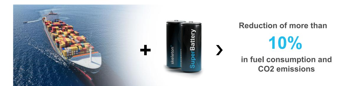
Today, all ships have a secondary generator that is being replaced with energy storage. 1-2 minutes of reserve available every 6 minutes is needed to ensure power availability and safety on board. Using SuperBattery energy storage to replace diesel generators reduces fuel consumption and carbon emissions by more than 10%, but also reduces noise, increases safety, takes less space, and requires no maintenance.
