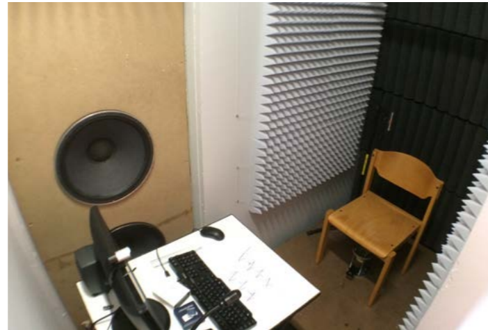
Figure 2 - Indoor low boom Simulator at University of Oldenburg, capable of reproducing the acoustic low-boom signatures and the associated vibrations.
