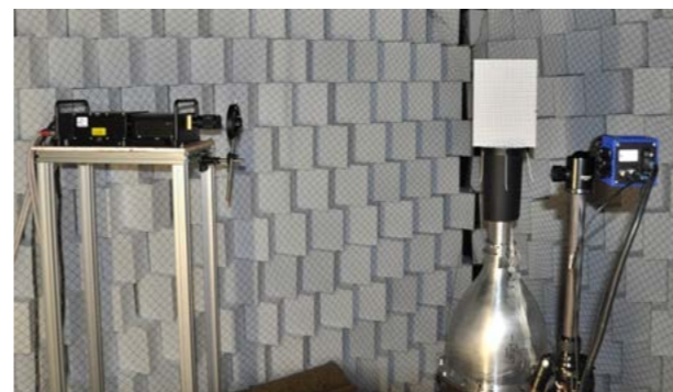
Figure 3 - Jet noise test campaign at the VKI anechoic facility JAFAR.
