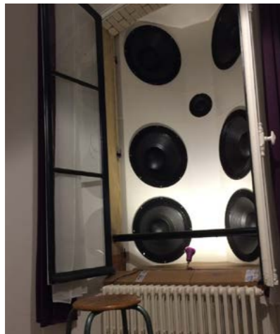
Figure 1 - Outdoor low boom simulator affixed to the window of a building at campus Saint Cyr of Sorbonne Université, capable of reproducing outdoor low booms within a test house.
