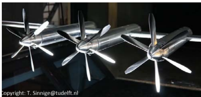
Figure 1 - Distributed electric propulsion model designed and tested at TU Delft, with adjustable relative phase between the propellers.
