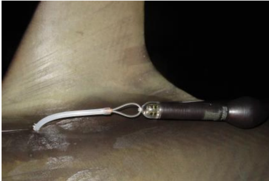
Figure 2. Photograph of a satellite PAT tag fixed in the dorsal musculature below the first dorsal fin of a pelagic shark.
