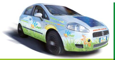
Mecaprom in the region of Piedmont, Italy, is fitting cars with hybrid-electric engines, batteries and solar panels.
