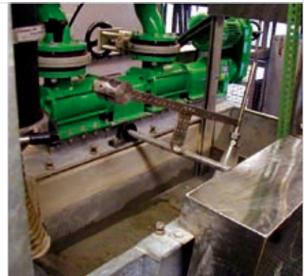
Jig for the wet treatment of the concrete sand fraction
