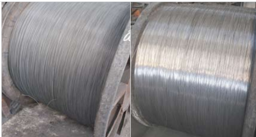
The absence of oxidation also gives the wire rod produced with the LIFE funded technologies a shinier appearance
