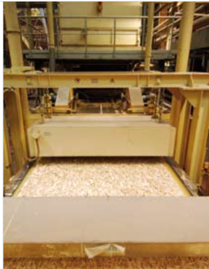
The ecoDry system captures VOCs before the wood flakes are processed into OSB panels
