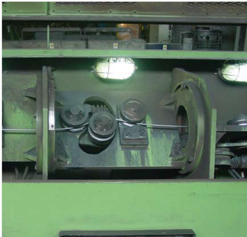
The innovative ESD rollers grind the wire removing 85% of the iron oxides
