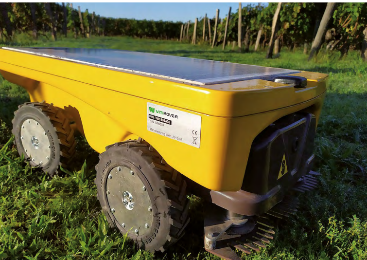
Vitirover mower robot used for vineyards
