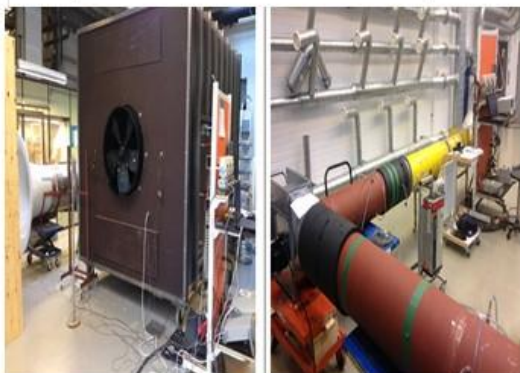
Category A and D methods of fan testing used in the INTAS project
