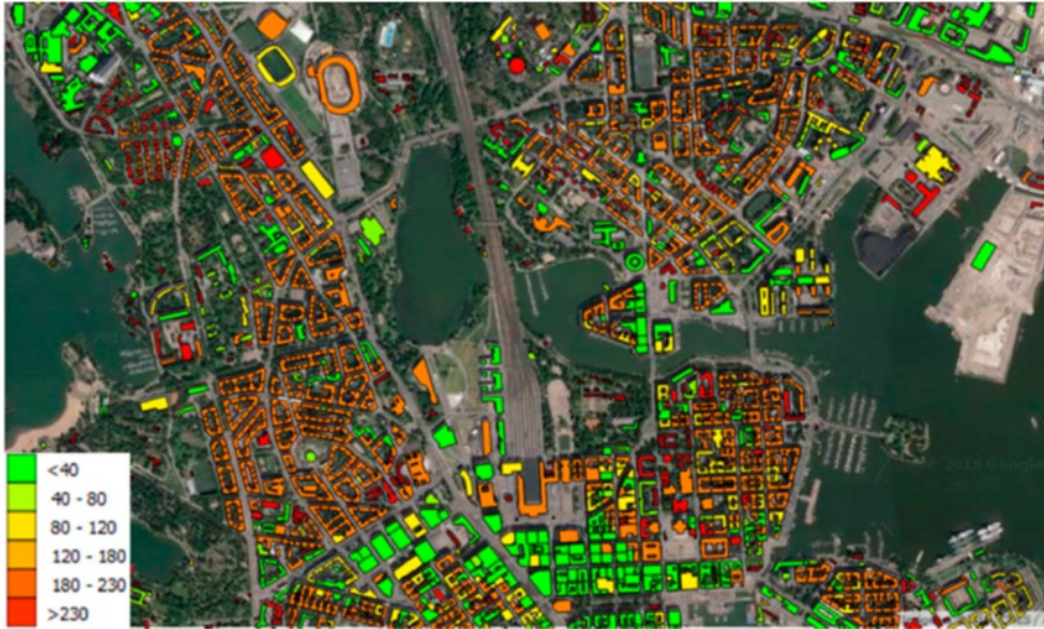
Figure 7 : Example modelling results for the heating demand (kWh/m 2 year) of the buildings of Helsinki [69].
