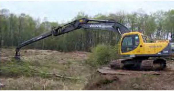
Machines used an 'island of plates' to cost effectively move around the wetland with minimal impact
