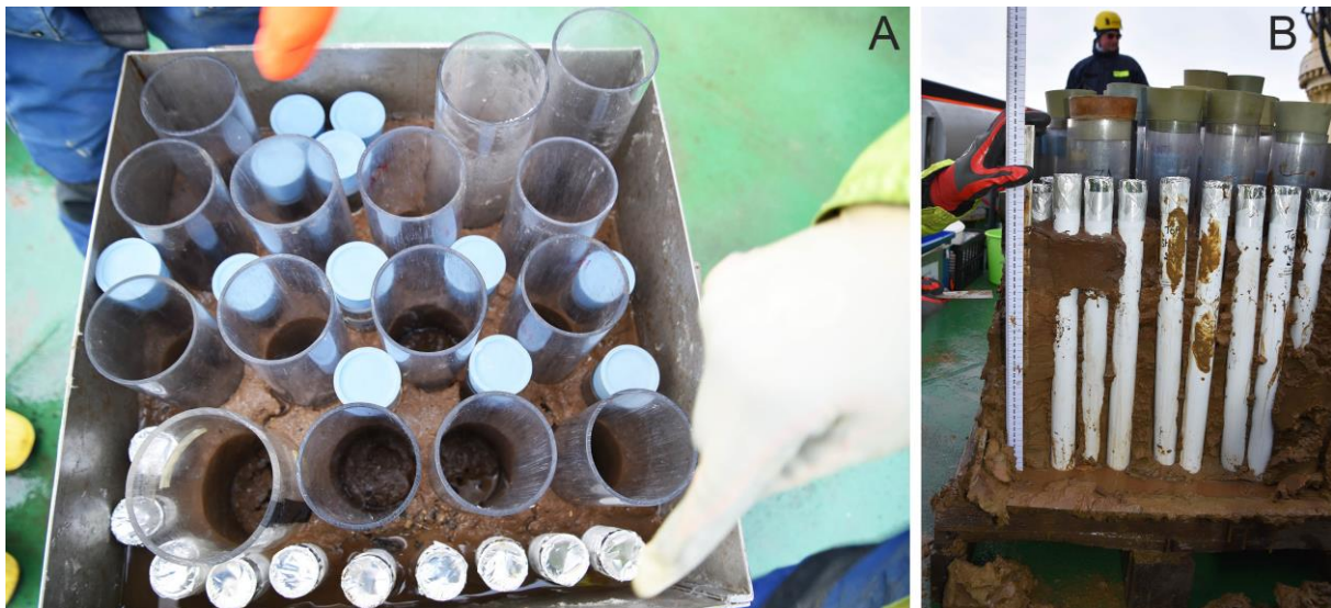
Figure 55: Subsampling a box core sample for Omics sediment samples during the SAS-Oden expedition. (A) Ten Omics samples were taken from each box core. (B) The Omics samples covered both the darker and lighter-coloured sediment layers (presumably the Holocene and interglacial layers) cf. Figure 47. (A,B) © Pauline Snoeijs-Leijonmalm
