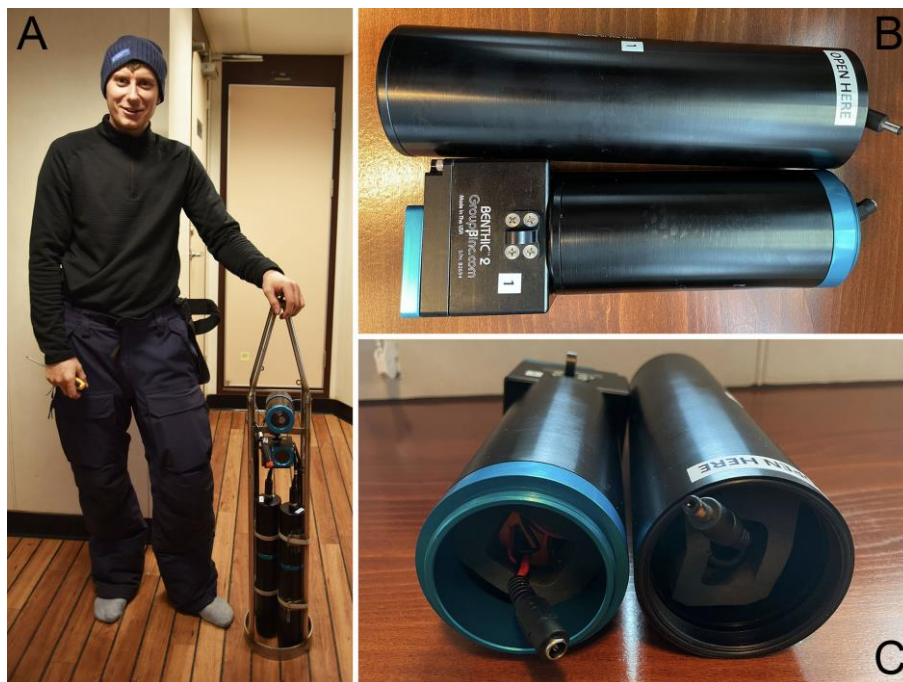
Figure 17: The Mini FishCam used during the SAS-Oden expedition. (A) Sideward-facing Mini FishCam on its stainless steel frame with the two battery tubes under the camera and the LED light above the camera. (B) Downward-facing Mini FishCam: camera and programming unit housing below the battery housing tube. (C) Downward-facing Mini FishCam: connection programming unit to the left and connection battery unit to the right. (A,B,C) © Pauline Snoeijjs-Leijonmalm
