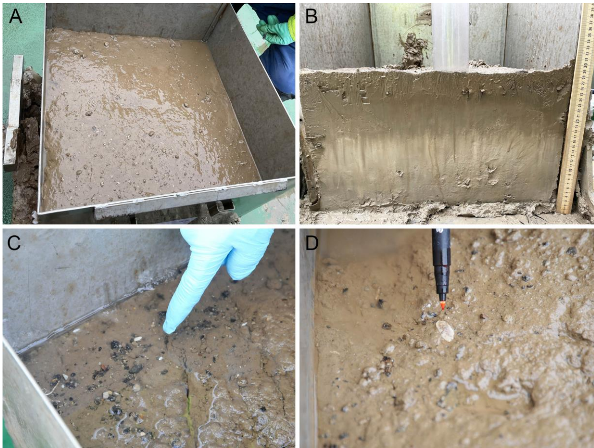
Figure 45: The structure of the box core samples taken during the SAS-Oden expedition – macroscopic animal life as almost absent. (A) The box core sample after removing the bottom water with silicone tubing. (B) The vertical structure of the sediment with the darker upper layer presumably representing the Holocene and lighter-coloured glacial sediment below it. (C) Otoliths were observed on the sediment surface. (D) The pencil is pointing at a relatively large otolith. (A,B,C,D) © Pauline Snoeijs-Leijonmalm
