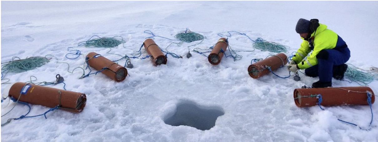
Figure 25: A deep trap line with six traps and a rectangular hole for deployment made by combining four 25-cm diameter auger holes in the ice. © Frank Menger
