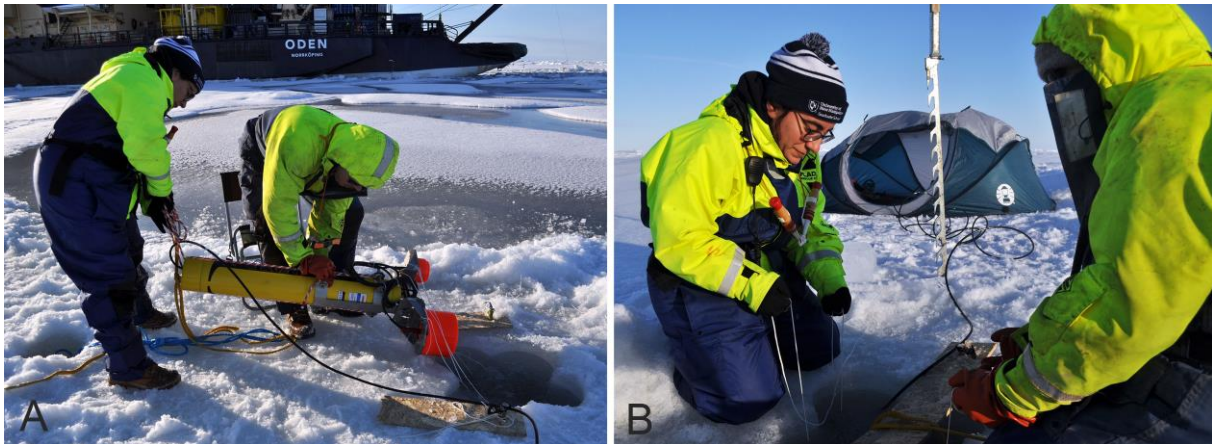
Figure 13: Calibration of the CTD WBAT used during the SAS-Oden expedition. (A) Preparing the WBAT for calibration on the ice at Station 58 (B) Manoeuvring the calibration spheres (A,B) © Serdar Sakinan
