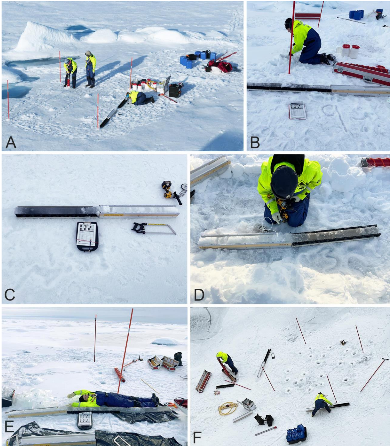
Figure 52: Ice coring during the SAS-Oden expedition. (A) A 5 x 5 m coring site has been selected and ice coring has started. (B) Measuring ice thickness through a coring hole. (C) Ice core in cradle with notebook, ice saw and drill. (D) Measuring a temperature profile in an ice core. (E) The longest ice core taken during the SAS-Oden expedition at Station 42, (F) Coring field after the coring had been completed. (A) © Johan Wikner, (B,C,D,E) © SAS-Oden sea-ice team, (F) © Pauline Snoeijis-Leijonmalm
