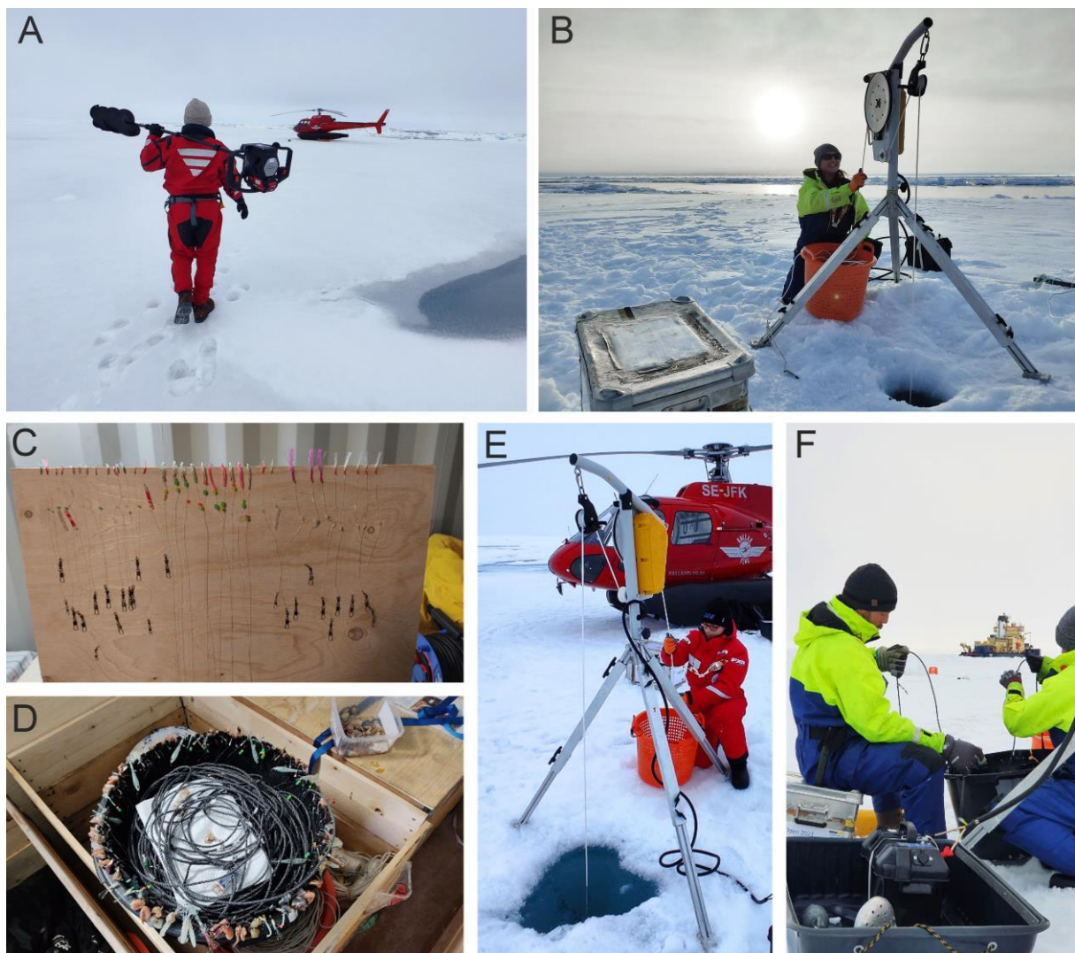
Figure 24: Deployment of longline. (A) Scientist carrying a 25-cm diameter auger used for making holes in the ice for the deployments during the SAS-Oden expedition. (B) A long line is hauled in with the help of a battery-driven winch on a tripod. (C) Hooks on a longline prepared for deployment. (D) Different hook sizes with artificial bait used for longline fishing. (E) The EFICA ice stations were reached by helicopter. (F) Line retrieval by hand-hauling. (A,B,C,D,E) © Frank Menger, (F) © Mats Persson
