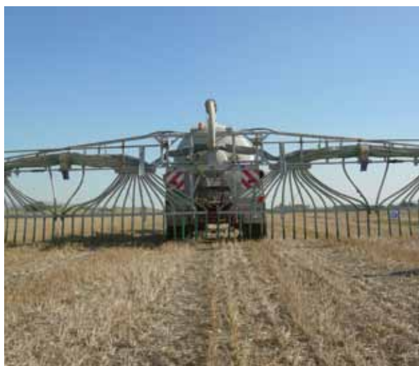
Trailing hose system for slurry application
