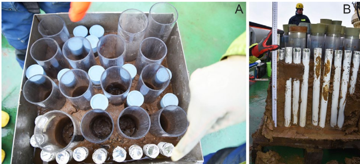
Figure 86: Sub-sampling a box core sample for Omics sediment samples during the SAS-Oden expedition. (A) Ten replicate Omics samples were taken with 10 white 3.8-cm diameter and 50-cm long polyethylene cores from each box core and immediately closed with aluminium foil on top. Twelve of the larger transparent plexiglas cores were used for benthic macrofauna and otoliths (WP6), and two were used for other projects. (B) The Omics samples covered both the darker and lighter-coloured sediment layers (presumably the Holocene and interglacial layers) (A,B) © Pauline Snoeijs-Leijonmalm
