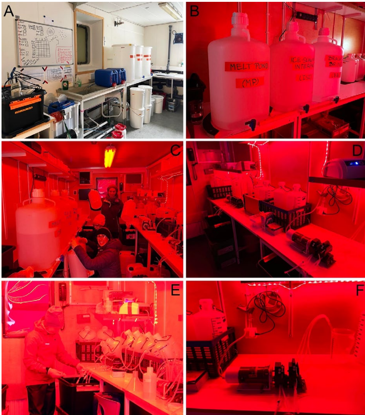
Figure 85: Omics filtrations in the red-light laboratory containers during the SAS-Oden expedition. (A) The 115-L containers for ice and snow. The snow was sampled in the white buckets and the top and bottom ice-core sections in the containers with red lids. Filtered seawater was available in the blue containers. (B) The 50-L containers with the ice-seawater interface, brine, and melt pond bulk samples. (C) collecting water from the bulk samples into 10-L bottles with scales to read the volume. (D) The peristaltic pumps used. (E) Filtration on Sterivex filters. (F) After the filtrations the peristaltic-pump tubing was rinsed with MilliQ water (A,B,C,D, F) © Pauline Snoeijs-Leijonmalm, (E) © Swedish Polar Research Secretariat (SPRS)
