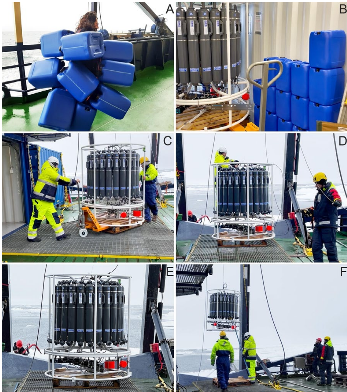
Figure 81: Preparations and deployment of the Omics CTD. (A) The blue 20-L carboys for sampling the Omics water are brought to the CTD container on the aft deck. (B) Carboys waiting for sampling the water. (C) The CTD is taken out of the container. (D) CTD prepared for deployment. (E) CTD ready for deployment. (F) CTD being deployed. (A) © Serdar Sakinan, (B,C,D,E,F) © Pauline Snoeijs-Leijonmalm
