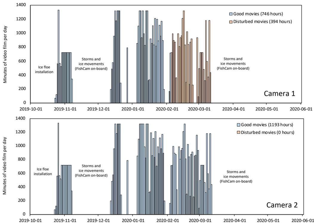
**Figure 5: Analysis of the number of days the two video cameras of the FishCam were recording video movies. The disturbed movies (orange bars) were due to a stray rope hanging in front of the side-ward looking Camera 1. This rope did not originate from the FishCam.**
