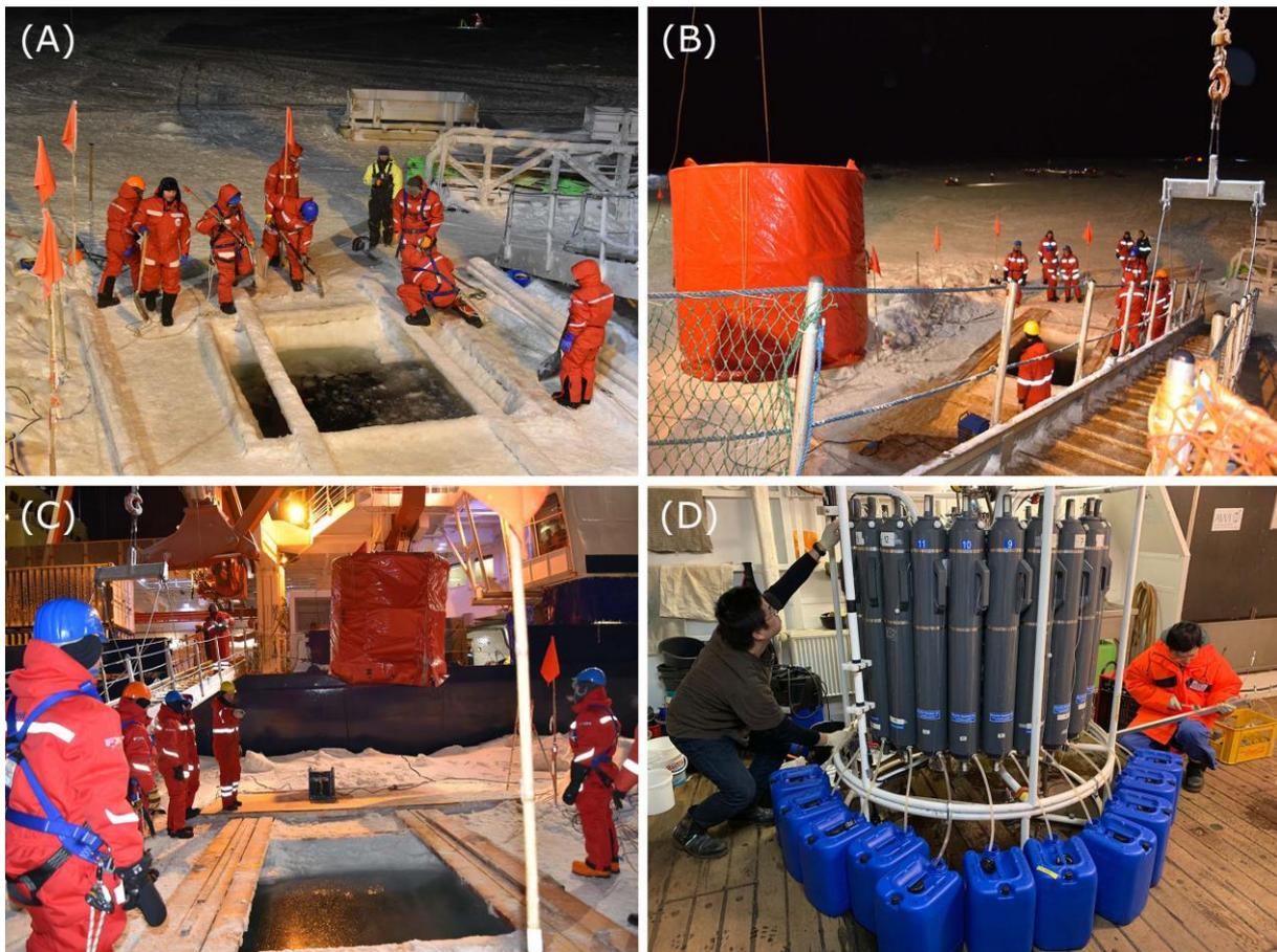
**Figure 51: Water sampling using a CTD rosette was not an easy task in winter. (A) The ice hole for the CTD next to the ship was kept open with chain saws and fin saws, and needed to be cleaned from floating ice with nets several times per week. (B,C) When the CTD was transported in air it was covered with a tent and heated. (D) Each of the 24 grey Niskin bottles could take a 12 L seawater sample at a pre-programmed depth. © Pauline Snoeijs-Leijonmalm (A-D), 2019**
