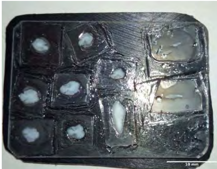
Figure 3. Glass slide with multiple samples to be placed on the laser chamber.
