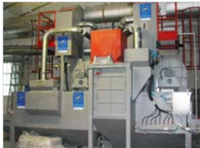
Traditional abrasive substances are replaced with the very same material used to make ceramic tiles
