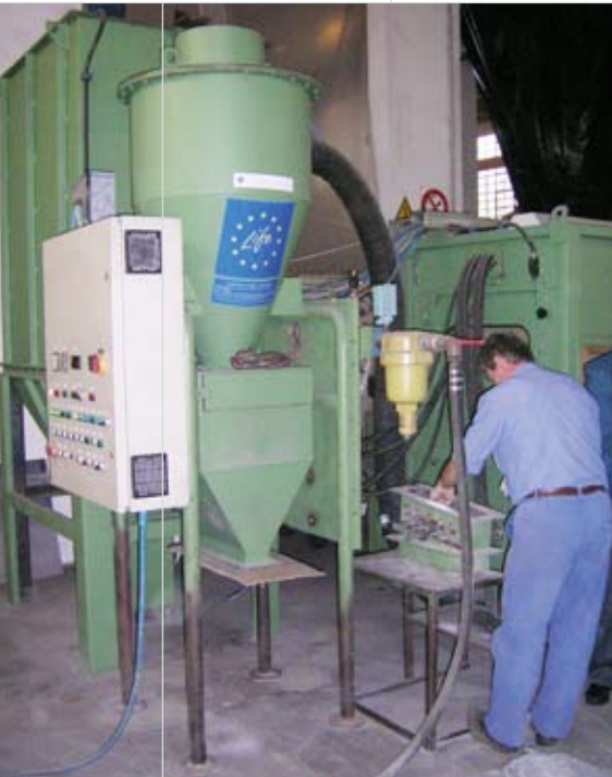
The abrasive material conveyance system is part mechanical, part gravity-powered and part pneumatic
