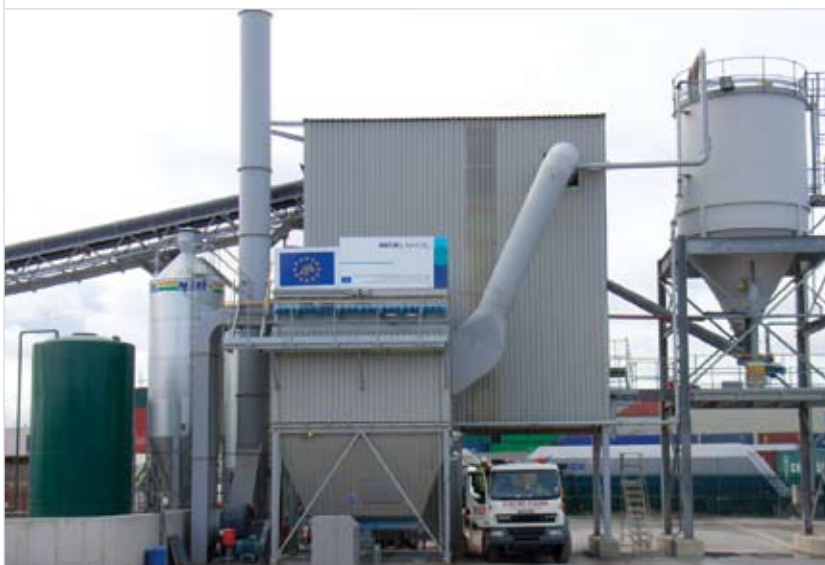
The modular unit developed by REF is shorter and takes up less space on the ground than traditional plants producing coated material
