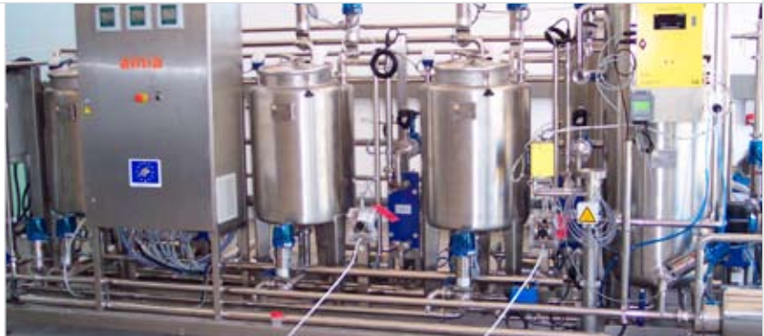
OzoneCIP went beyond the current BAT by using ozone as an alternative cleaning agent in a clean-in-place system
