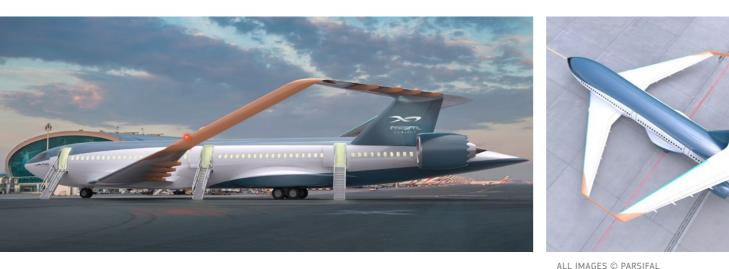
The PARSIFAL project is designing a disruptive box-wing aircraft, called the "PrandtlPlane". The novel design of the PrandtlPlane demonstrated notable aerodynamic advantages since it is capable of minimizing the induced drag for a given total lift and wingspan.
