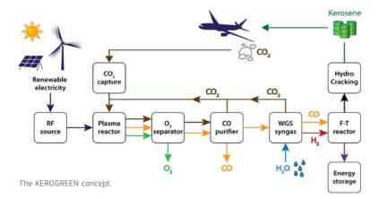
The KEROGREEN approach meets the ICAO CORSIA emission reduction objectives and the Flightpath 2050 environmental objectives, as this fuel contains no sulphur, produces no soot and reduces NOx emissions. This CO<sub>2</sub>-neutral Power-to-X technology strengthens the EU energy security by creating a long-term, large-scale storage capacity, and is generic in coupling the power sector to other fuel and chemical driven sectors.
