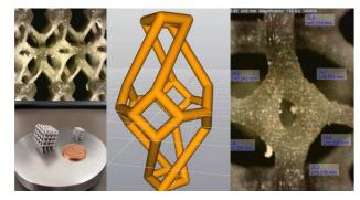
The AERIALIST project disclosed the potential of metamaterials in aeronautics through four pillar actions: i) consolidated the aeroacoustic theory of metamaterials; ii) developed and assessed methods for efficient additive manufacturing of metamaterials; iii) validated models and design through wind-tunnel experiments; iv) assessed the entire toolchain loop modelling-manufacturing-experiments and provided a development roadmap towards TRL of industrial relevance.
